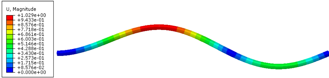
(b) The second order mode shape of FEM.
